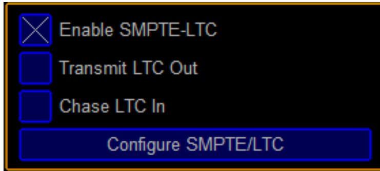
Linear Time Code (LTC) is an audio signal which contains time code information. TimeLord can send or receive LTC using standard audio interfaces (headphone socket and microphone socket on a laptop for example.) You can share your default audio device if you only have one, and produce LTC on one channel and media audio on the right channel. Many devices support LTC, and you will probably need an 3.5mm to 1/4" jack or XLR adapter to connect to professional equipment (ask the audio guy).
