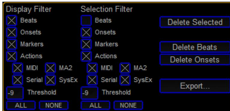
These tools affect which events are displayed in the Wave Form window, and which events can be selected by the mouse. Pressing “Delete Selected” does exactly that, and “Delete Beats” and “Delete Onsets” can be used to remove all DSP introduced events.
