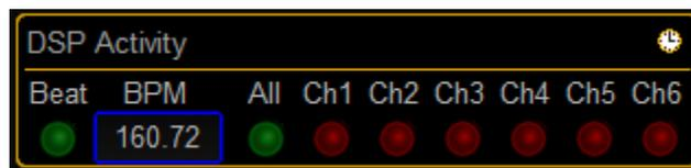
**Clicking** on one of the red LED's will present an Event Editor that you can assign an event to a channel for a cue. Ch.1 is loudest onsets and Ch.6 is softest onsets, and Beat is the Beat. This allows for sending MIDI or MA2 commands every time the channel becomes active, which can trigger a light or sequence for example.
